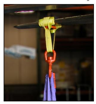
Lift-All's new patent pending *GripHook* design converts your fork truck into an overhead lifting device in a matter of seconds. This is a must for contractors, manufacturing plants, power plants, distribution centers, rental houses, and any other facility using fork trucks.
